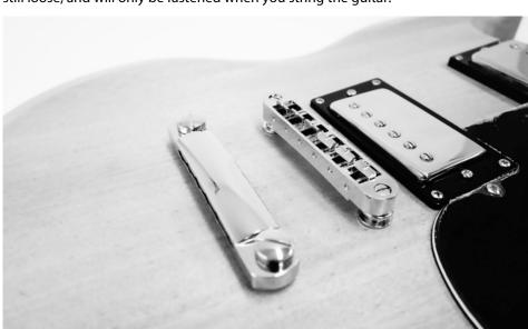
Place the tailpiece and the bridge on the fastening bolts. These two components are still loose, and will only be fastened when you string the guitar.
