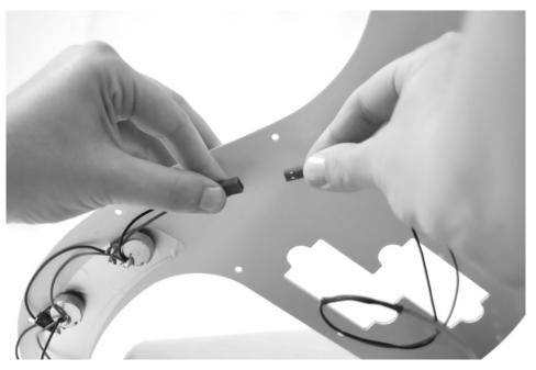
Connect the connector to the connector for the potentiometers and output jack which is mounted on the pickguard.
