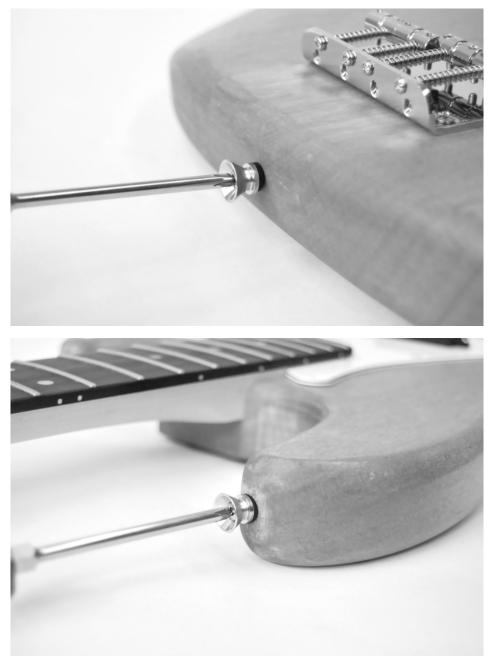
Screw the strap buttons into the pre-drilled holes in the body as shown.
