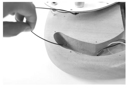
Run the cable for earthing the strings (stripped, without connectors) through the channel in the recess for the potentiometers and into the hole on the front.
