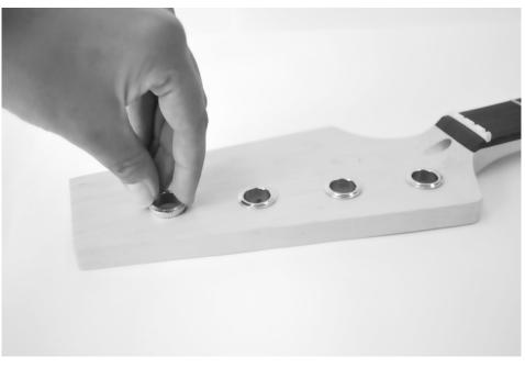
From the rear side of the headstock, insert the tuners into the holes provided. Align the tuners so that the tuning pins are vertical to the upper edge of the headstock.
