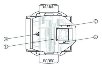
**9.** Reattach the illuminant cover and secure it with the two Phillips screws (marked in the illustration by 'C').
