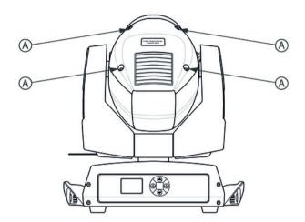
Open the housing by unscrewing the four Phillips top screws marked in the illustration above by 'A' and remove the upper part of the housing. Make sure that no screw falls inside the unit.
