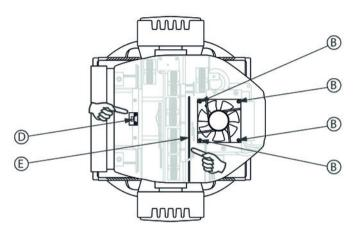
Check that you have removed the proper cover. Compare the exposed interior of the unit with the illustration. If you can see the heat sensor (marked in the illustration by 'D') at this point, the proper side of the case has been opened. If the correct side of the case is open, you can also clearly see the colour wheel (in the figure marked by 'E').
