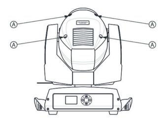
Put the upper part of the housing back on the base. At that point, both housing parts must engage in the circumferential seal profile. Replace the four Phillips screws ('A') to the top of the housing and tighten them.
